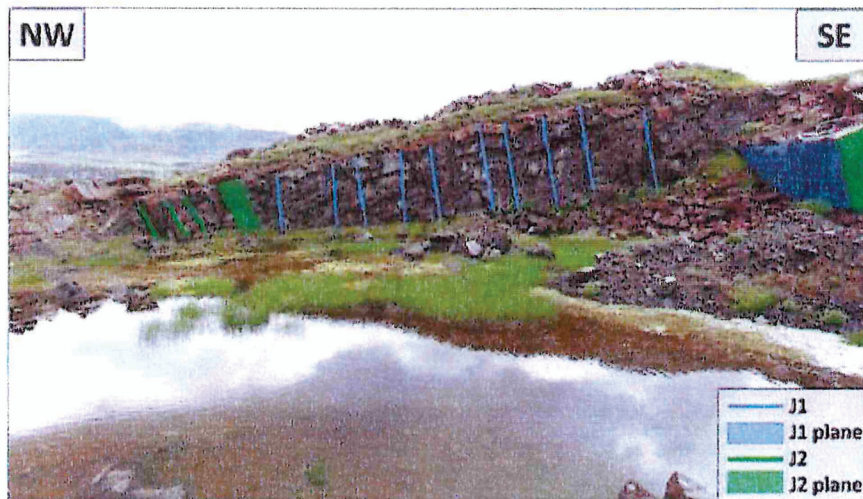
Figure 6 a-c: Joints and joint planes of both J1 and J2 observed in the study area.
