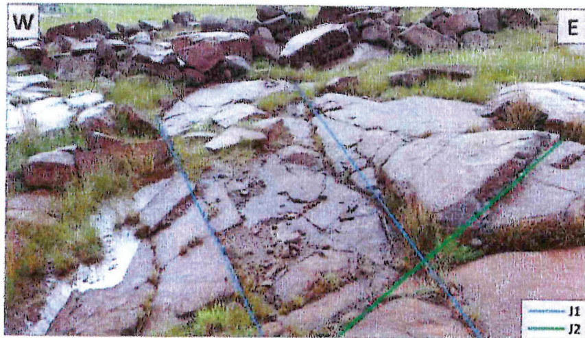
Figure 7 a-b: Joints observed in solid dolerite outcrops in the surrounding study area.
